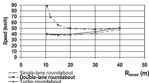
Fig. 1. The impact of the type of a circular intersection on the vehicle speed (Fortuijn, 2009).
