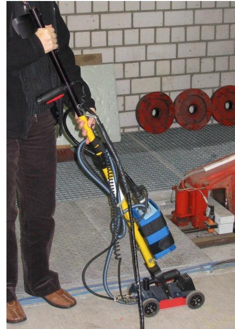
Fig. 3 - 1,5 GHz GSSI dipole antenna: measuring in test pit
