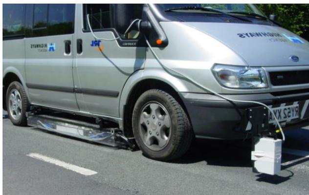
Fig. 6 - Four-channel system used in TRL: attachment to measuring car Harris (photo TRL)
