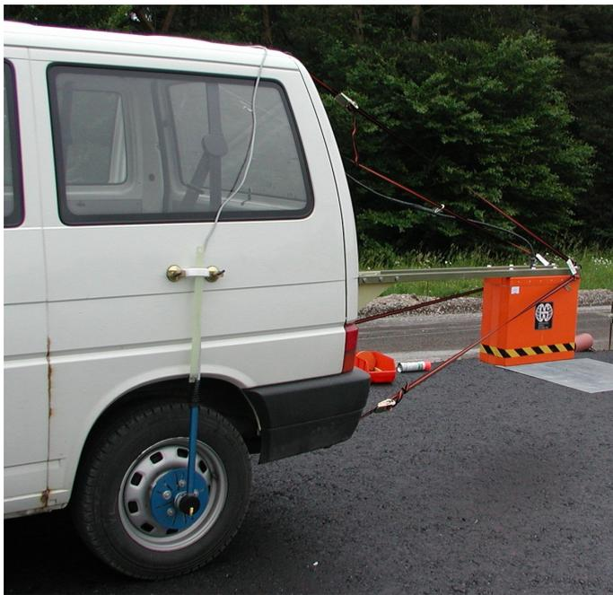
Fig. 2 - 2 GHz GSSI horn antenna: attachment to the measuring car
