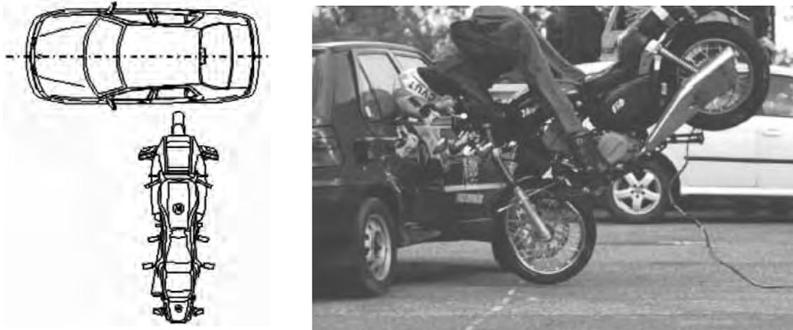
**Figure 8a, 8b: Experimental simulation in impact configuration 413 according to ISO 13232 [2]**
